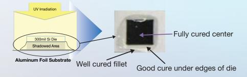
Shadow curing is often critical to designs where access to UV light is limited
